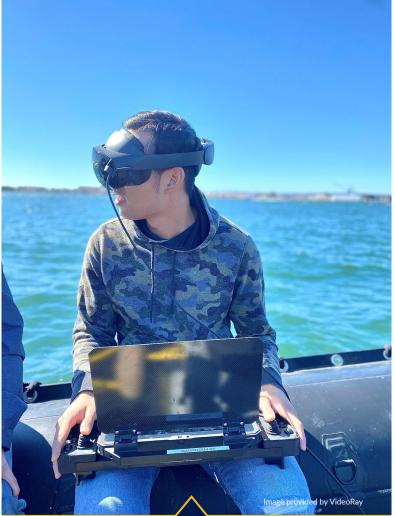
Blue Ring's mixed reality software application for ROV control runs on a head mounted display (HMD) ruggedized for outdoor use.
